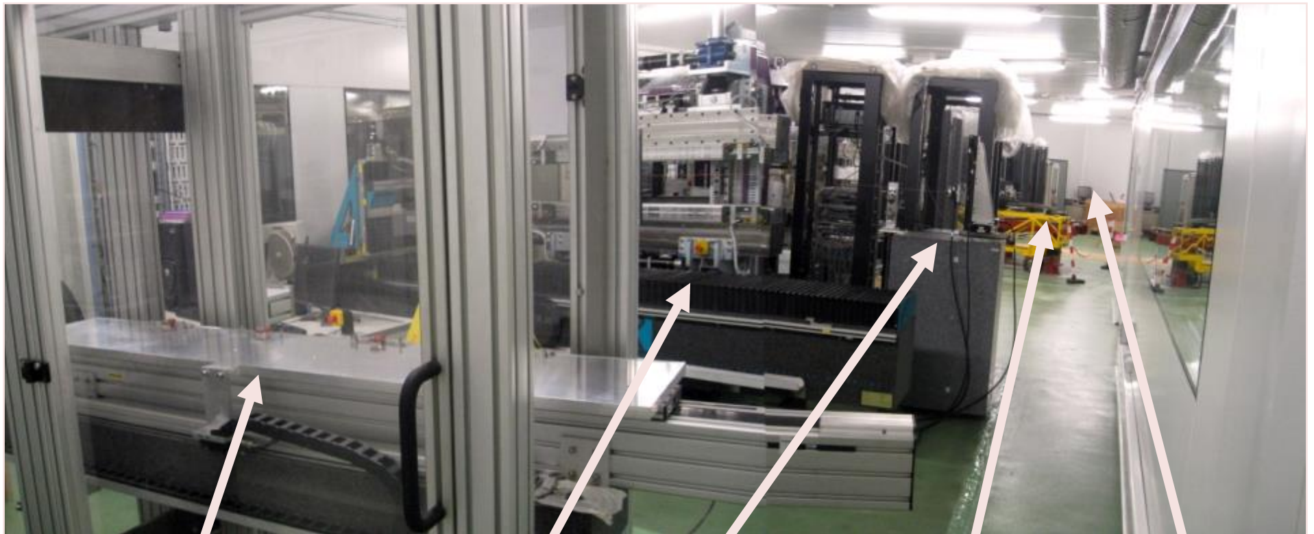
Fixed stretched wire bench
