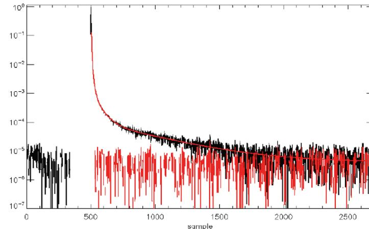
Thermal modeling is important. Long time constants might come from the links between the wafer and the detector housing and are seen on both categories of glitches
