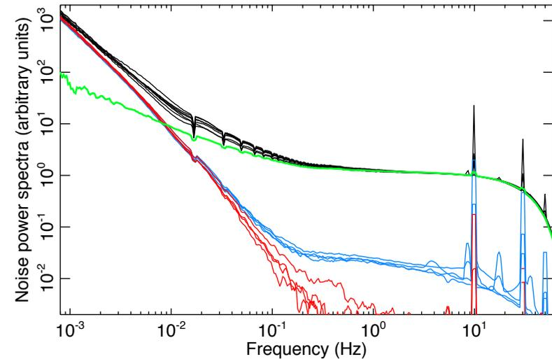
Data acquisition locked on the 4K cooler compressor: fixed line frequencies, multiple of 20 Hz (before demodulation)
