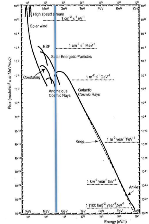
Cut off due to material around the detectors at  $\sim 50$  MeV
