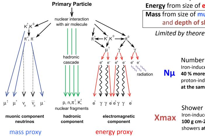
Direction from particle arrival times Energy from size of eγ component Mass from size of muonic component and depth of shower maximum
